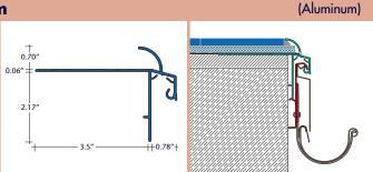
It is designed to protect the edge of the tile installed over our underlayment, and to cover the edge of the exposed balcony/terrace substrate. The profile features an overhang extension deflecting water running off the tile installation from the balcony substrate. This extension can also hold additional components of the Blanke®BALCONY System including the gutter holder and gutter shield. Drainage holes allow for run off of moisture collected by the drain mat system.
